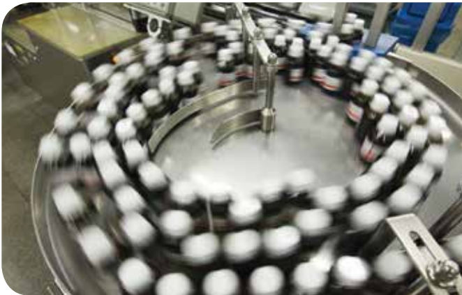
42JT - Detecting Presence of Bottle Cap in Packaging
